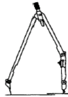
(b) Position of the lead leg to draw larger circles
