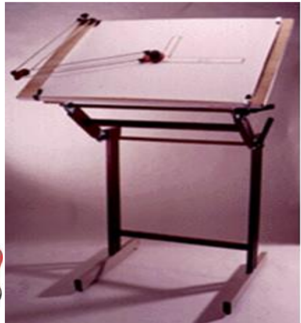
Fig 1.5 Drawing Board and Mini Drafter Assembly
