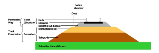
The rails are joined in series by fish plates and bolts & they are fixed to sleepers by different types of fastenings. The sleepers properly spaced, resting on ballast are suitably packed and boxed with ballast. The layer of ballast rests on the prepared sub grade is called as the formation.
