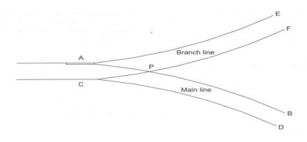
(**Fig:** Negative superelevation)
