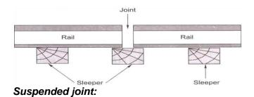
In this type of joint, the ends of the rails are suspended between two sleepers and some portion of the rail is cantilevered at the joint. As a result of cantilever action, the packing under the sleepers of the joint becomes loose particularly due to the hammering action of the moving train loads. Suspended joints are the most common type of joints adopted by railway systems worldwide, including India.
